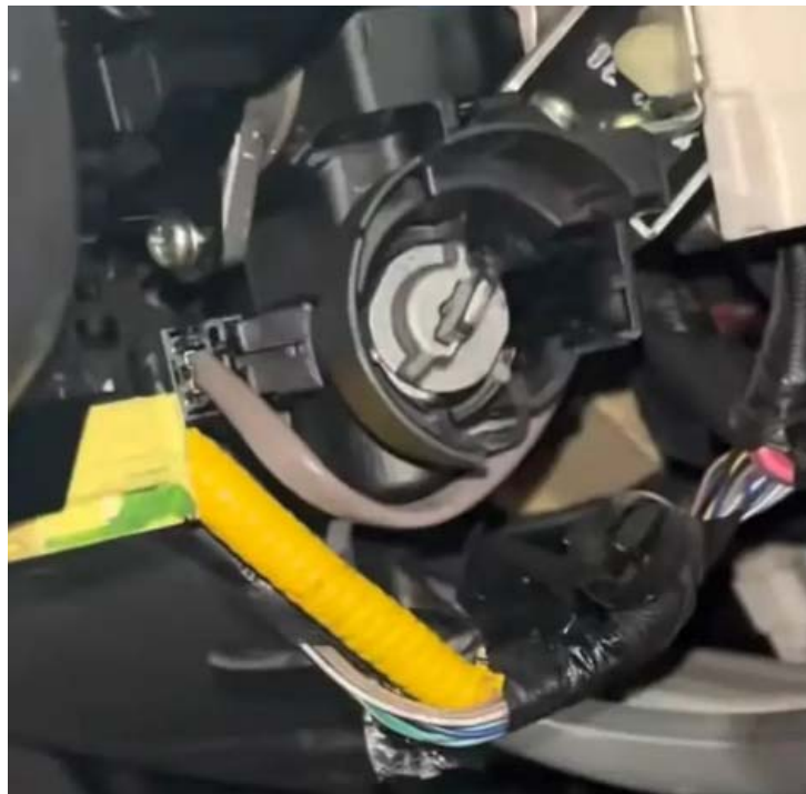
Exposed ignition switch spade after ignition cylinder is removed
