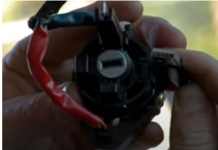
Exposed female port at the back of ignition cylinder
